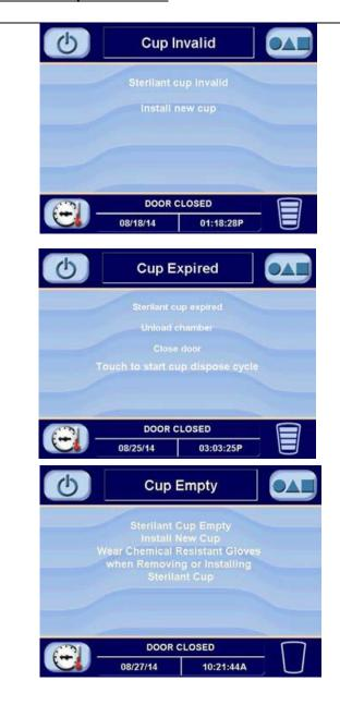
The following displays shall appear to prompt the use to install a new sterilant cup
