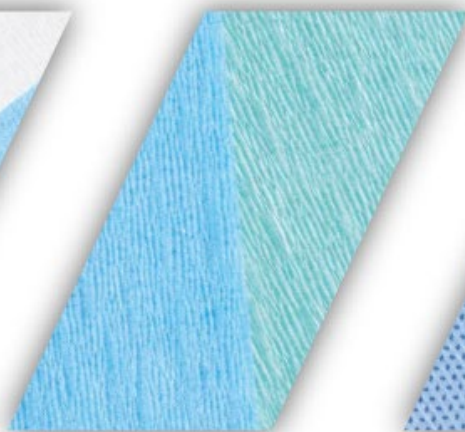
WETLAID NONWOVENS cellulose + synthetic fibers
